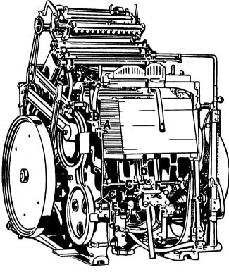
Control A starts and stops feeding of stock. Control B regulates the air blast for different weights of stock.
